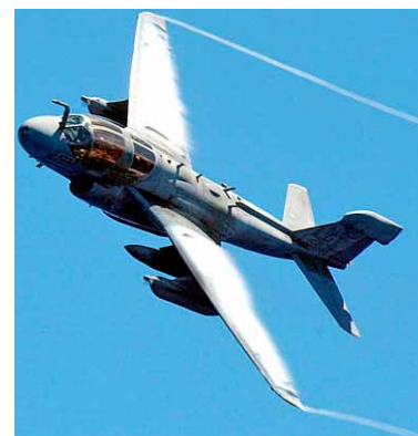
Fig. 3. Condensation in the core of the wing tip vortices of an aircraft (source: United States Navy 2003)
